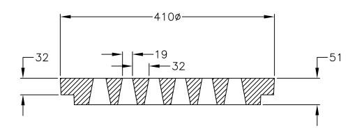
DESIGNED TO FIT THE BELL END OF 15" (375MM) CONCRTE PIPE
